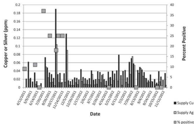
**Fig 4.** Copper and silver ion concentrations during start-up and stabilization of copper-silver ionization. Superimposed on the bars are the corresponding percentages of positive cultures (light gray squares). Early low transients (July, October, and November 2011) resulted in rapid increases in positive cultures, whereas later transients did not (April, July, and November 2012).
