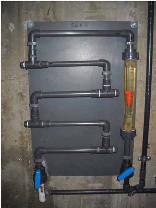
FIG 1 Example of a rack used to support coupons for the test of corrosion.
